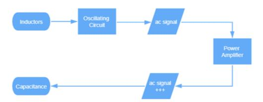
The resonant coupling technology uses two resonant objects of the same frequency to create a strong mutual coupling, with the energy interacting between the two objects, using the coils and the flat capacitors placed at both ends to form a resonant circuit. The voltage transmitted to the car is processed by the circuit to supply the motor and to store the capacitor.
